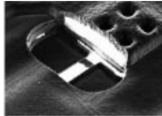
Blown polysilicon fuse near test pad (Motorola)
